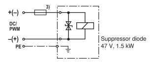
3) Recommended pre-fuse characteristics: medium time-lag according to DIN 41571, 1.25 A
